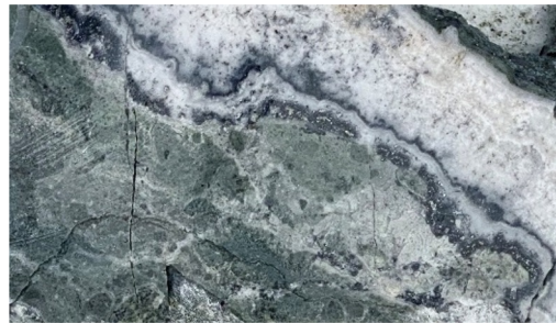
2 Ginguro banding in drill core from CDH-001 (3.00 m @34.7 g/t gold, 3,129 g/t silver from 111 m).
